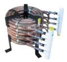
Edwards "5VS" series double wall vented tube heat exchanger with Titanium water tube & copper outer refrig tube for Aquaculture water heating.
